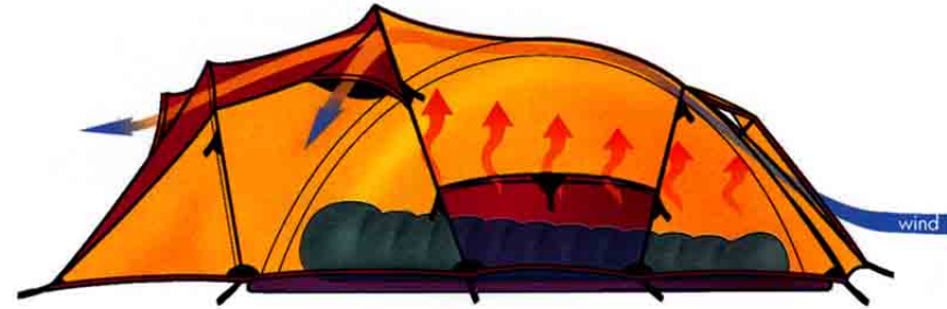
Double Wall Active Ventilation
