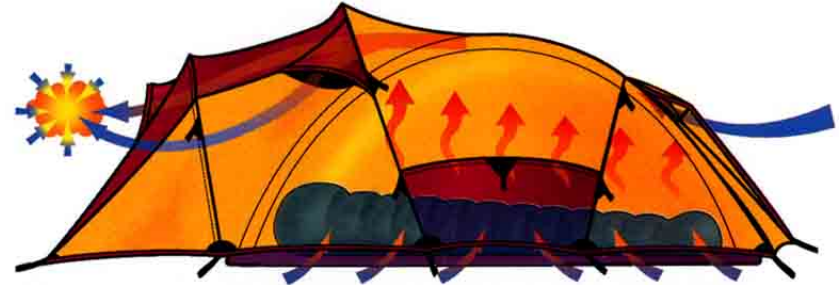
Double Wall Passive Ventilation
